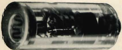
Fig. 6 - Come si presenta il cablaggio dopo la colata. A black and white photograph showing the same complex arrangement of wires and components as in Fig. 5, but now enclosed in a cylindrical metal housing.
